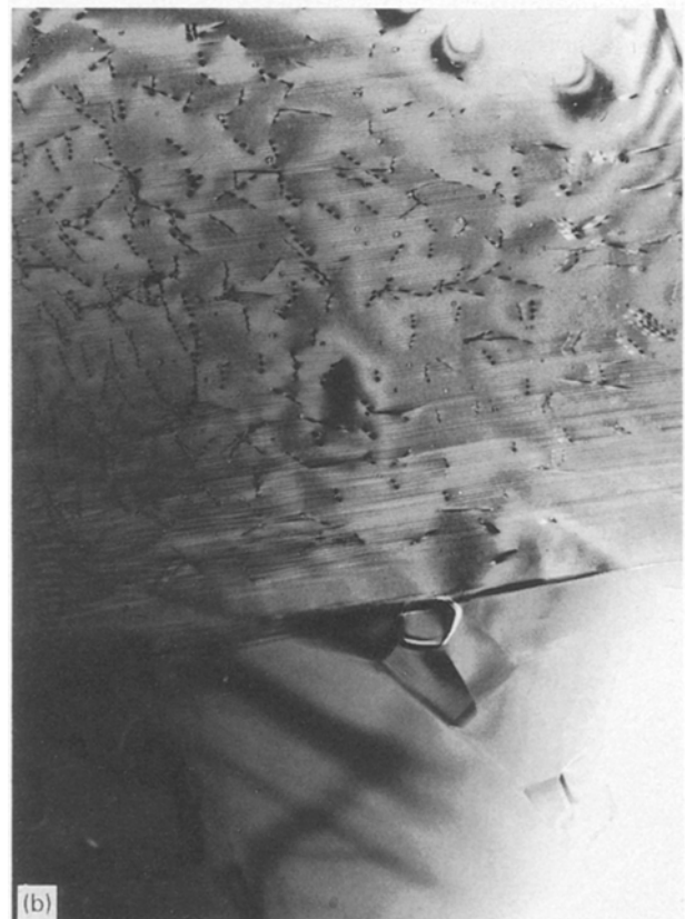
Figure 15 Planar defects in SiC platelets after sintering observed by TEM at different tilt angles.
