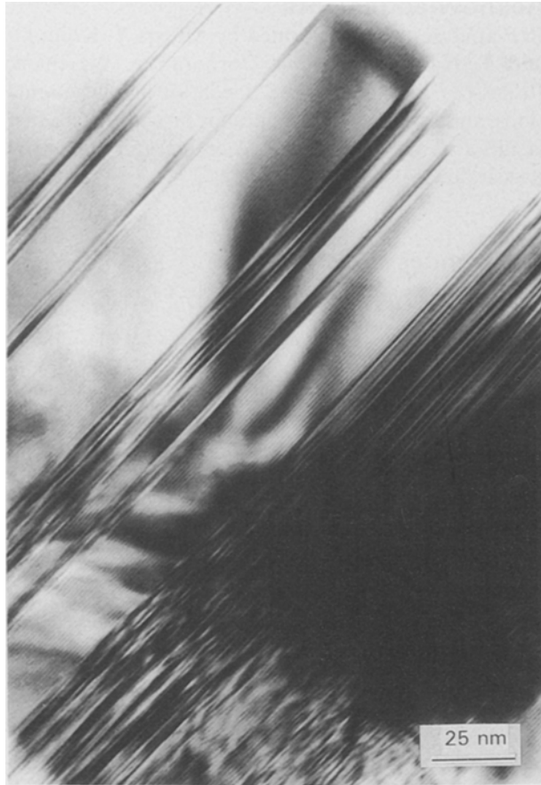
Figure 14 Low-magnification TEM image of a SiC platelet showing a low density of stacking faults.
